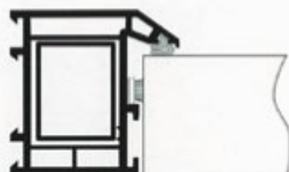
70mm PVCu reinforced outer frame
